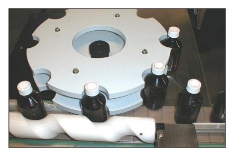
The Model 3892 utilizes a Timing Screw Drive Unit to acquire positive control of the container prior to entering the Vacuum Reject Starwheel. The Drive Unit and Starwheel are mechanically linked together to ensure correct timing between both units.
